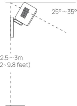
On a masonry surface (3M tape can be used to fix the position before screw driven in)
