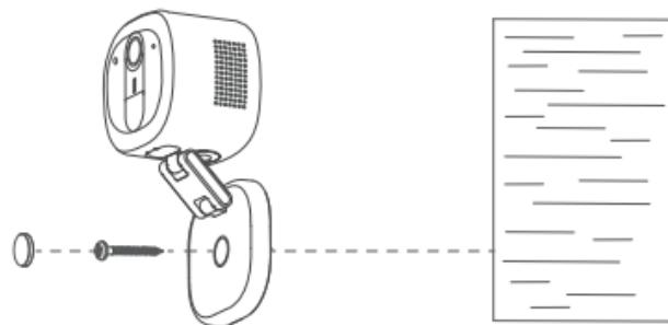
■ Install on the ceiling (3M tape can be used to fix the position before screw driven in)
